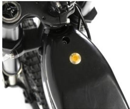
65% and red when the battery charge reaches 30%. The red light will start blinking when the battery charge is very low. From this point, the bike will start losing power and will be able to travel roughly 2 – 3 km (1 – 2 miles) before the motorcycle shuts down completely.
